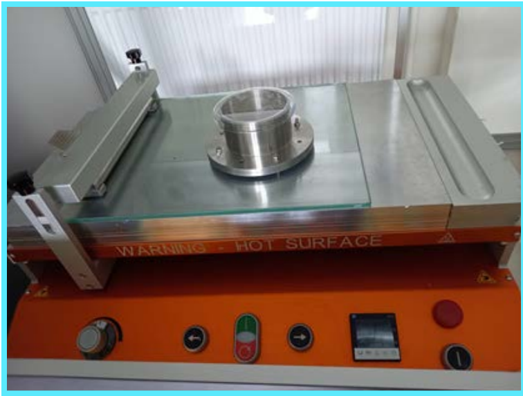
Casting table for the deposit of the thin layer on the support
