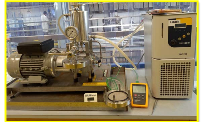
Reverse osmosis setup for membrane testing
