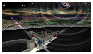
Telescope will achieve a greatly improved sensitivity by increasing the size of the interferometer from the 3km arm length of the Virgo detector to 10km, and by implementing a series of new technologies. These include a cryogenic system to cool some of the main optics to 10-20K, new quantum technologies to reduce the fluctuations of the light, and a set of infrastructural and active noise-mitigation measures to reduce environmental perturbations.
